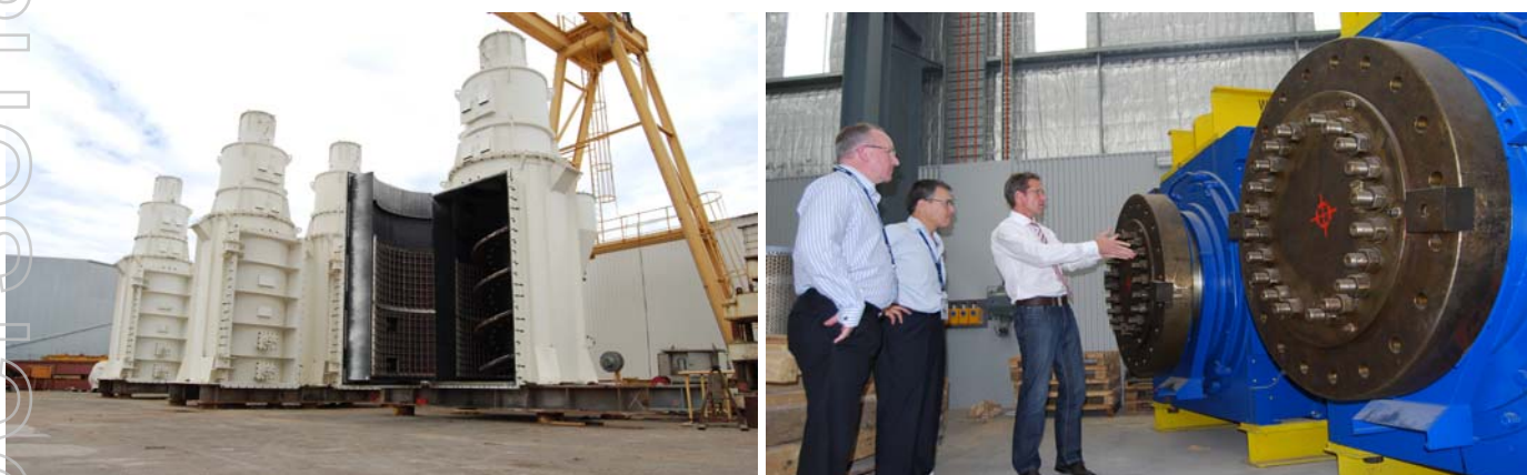
Four tower mills (L) have been completed and being stored in Perth. Steve Murdoch (KML chief operating officer) and Garret Dixon (Gindalbie managing director) view progress on Karara's high pressure grinding rolls (R) being supplied by Thyssen Krupp.
